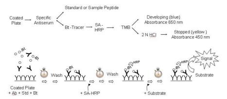
This ELISA kit is a competitive immunoassay. The antiserum is captured by antibodies coated on a 96-well plate. A constant concentration of Bt-tracer (biotinylated tracer) and varying concentrations of unlabeled standard or sample peptide compete for binding specifically to the antiserum. Captured Bt-tracer is subsequently bound by streptavidin-conjugated horseradish peroxidase (SA-HRP), which produces a soluble colored product after a substrate is added.
